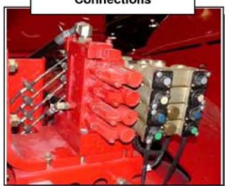
Hydraulic Valves / Couplers Assembly with Standard Mechanical Remote Control Connections
